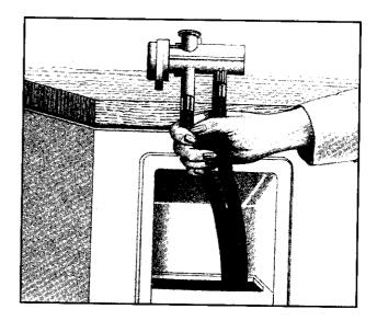
Press down on thumb release. Lift connector up on to faucet and remove pressure from thumb release to hold connector firmly in place.
